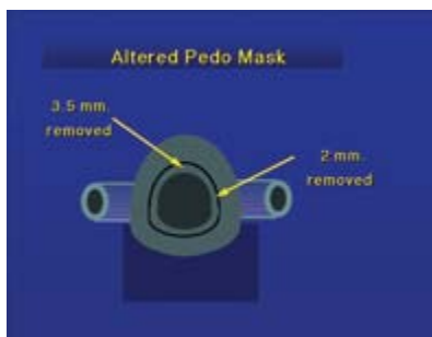
Figure 13. By altering the shape and size of the nose hole, a pediatric mask can be used by adults.
