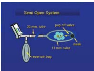
Figure 6. The semi-open system allowed gas to escape from a pop-off valve on the mask and into the breathing space of the dentist and dental assistant. This led to nitrous oxide levels as high as 5,000
