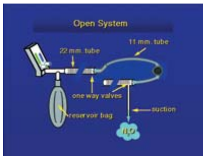
Figure 11. In the open system, gas is drawn from the bag and exhaled through a second hose, or into a space around the mask. Suction then removes the waste gas.
